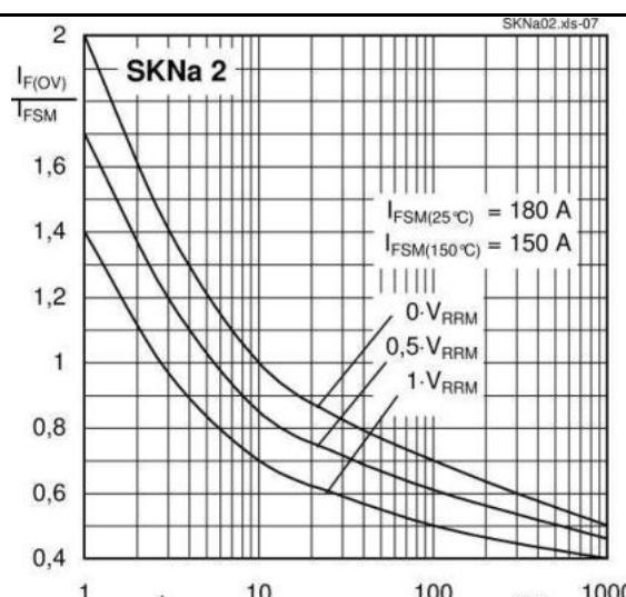
Fig. 6 Rated surge overload current vs. time
