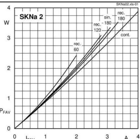
Fig. 1 Power dissipation vs. forward current
