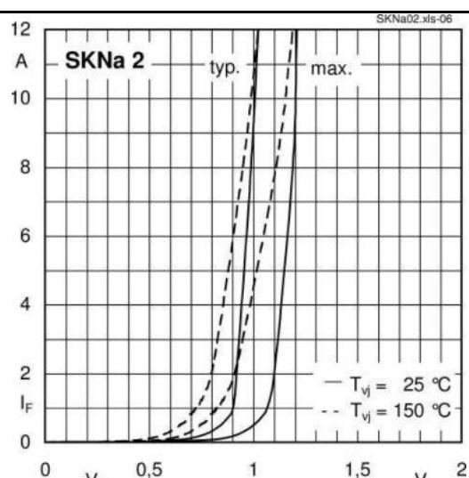
Fig. 5 Forward characteristics
