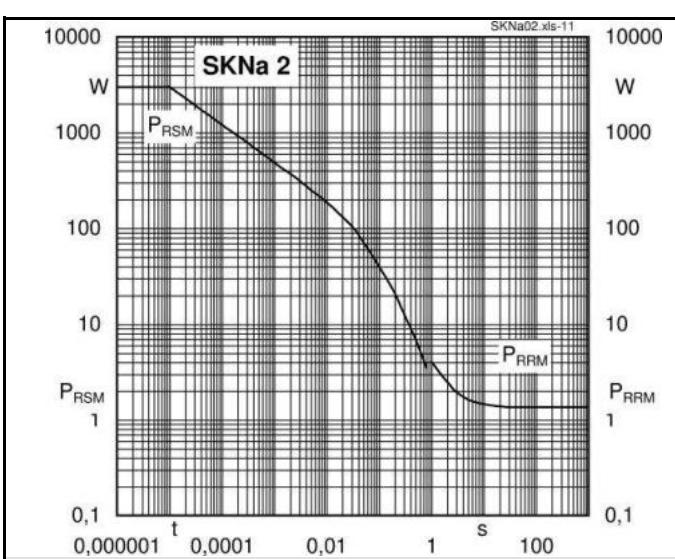
Fig. 9 Reverse power dissipation vs. time
