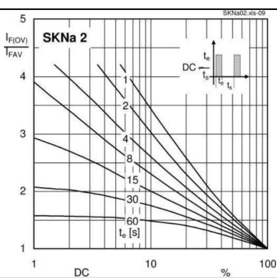
Fig. 7 Rated overload current vs. duty cycle
